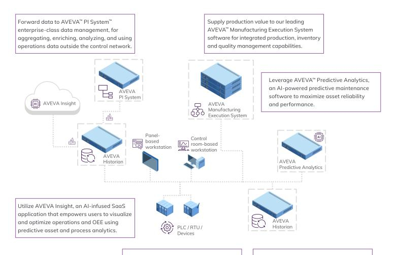
Connect to new and existing HMI/SCADA, PLC/RTU, and other third-party sources for data capture and preservation.
